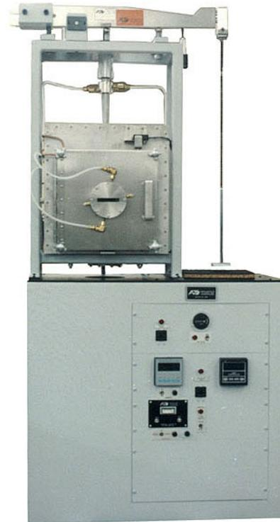
*Series 2390 Compression Creep Tester modified for high-temperature flexural static fatigue testing of continuous fiber-reinforced ceramic composites (CFCCs) in a controlled-atmosphere environment.*
