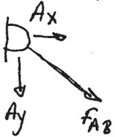
note that the pin reactions at A have the resultant of  $F_{AB}$ , directed along the axis of the bar:  $F_{AB} = \sqrt{A_x^2 + A_y^2}$
