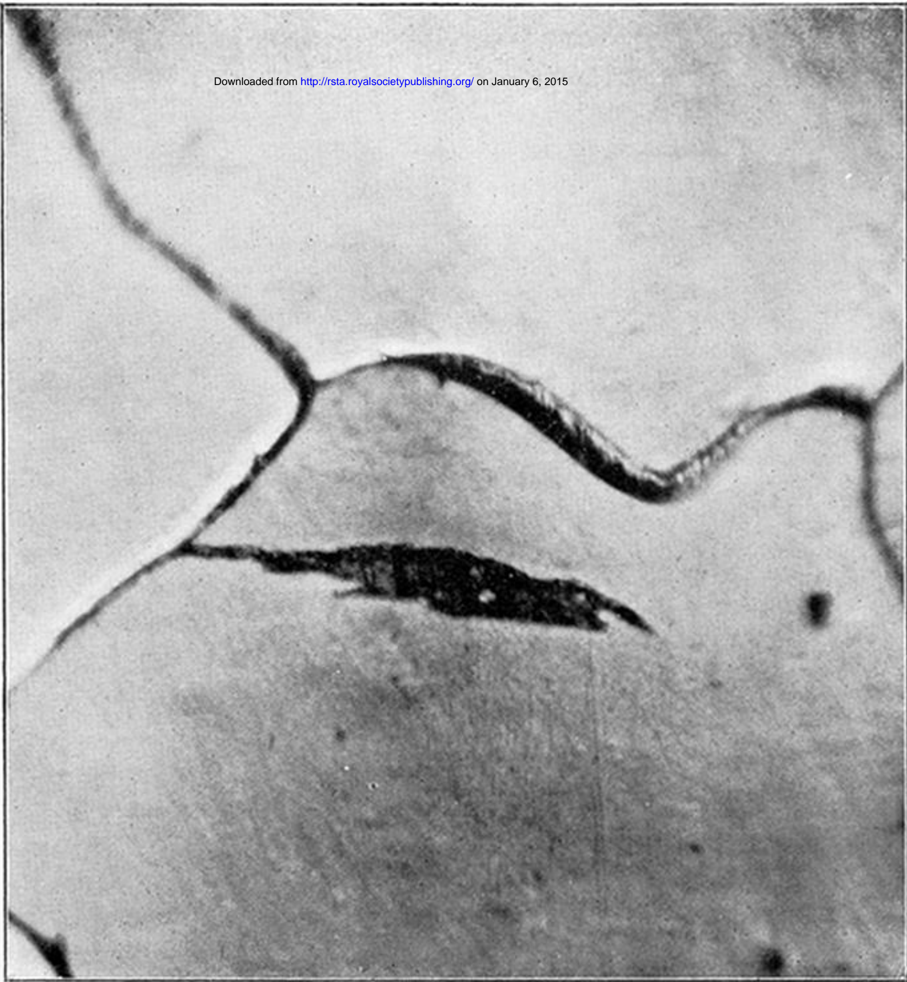
Fig. 15. Specimen after 3,000,000 reversals of a stress of 6·9 tons per sq. inch. \times 1000 .
