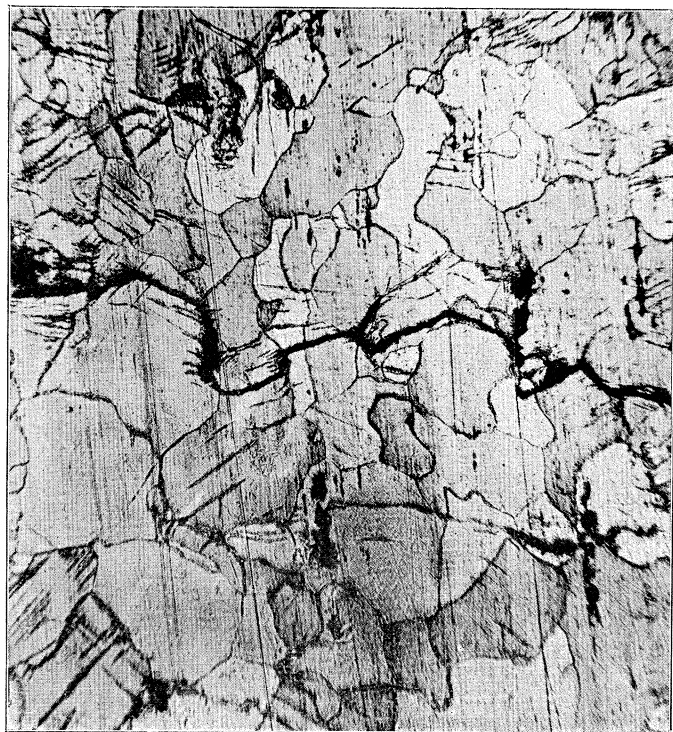
Fig. 7. Specimen after 170,000 reversals of a stress of 12·3 tons per sq. inch. \times 150 .
